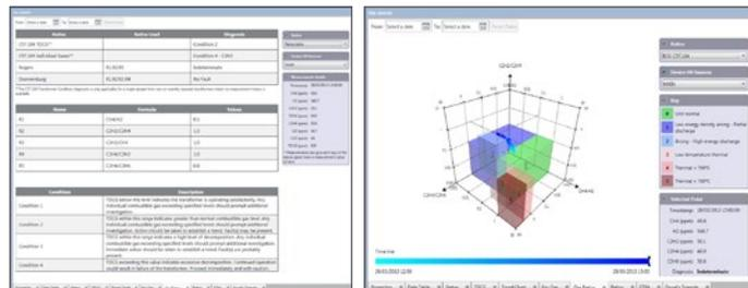
Encompasses the IEC 60599 & IEEE C57.104 standards in a 3D rotatable graph. Rogers and Doernburg ratio diagnostics are also included in a separate concise and detailed table.
