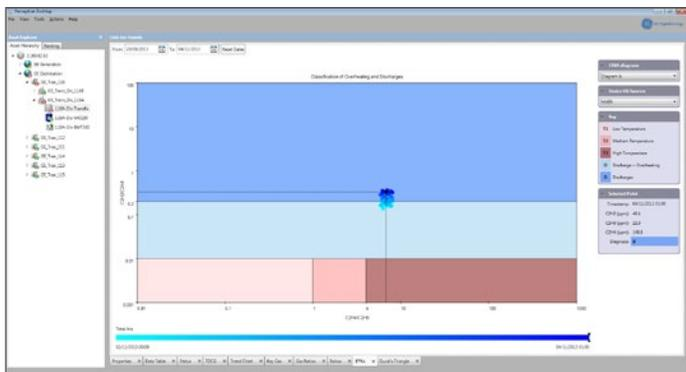
Diagrams A and B compare concentrations of  $C_2H_2/C_2H_4$  against  $C_2H_4/C_2H_6$ , as well as  $C_2H_2/C_2H_6$  against  $C_2H_4/C_2H_6$  in order to determine fault conditions.
