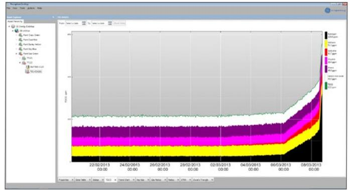
Displays the total dissolved combustible gas as relative concentrations within a trend chart. This view allows the user to quickly gauge the relative ratio concentrations of the individual gases.
