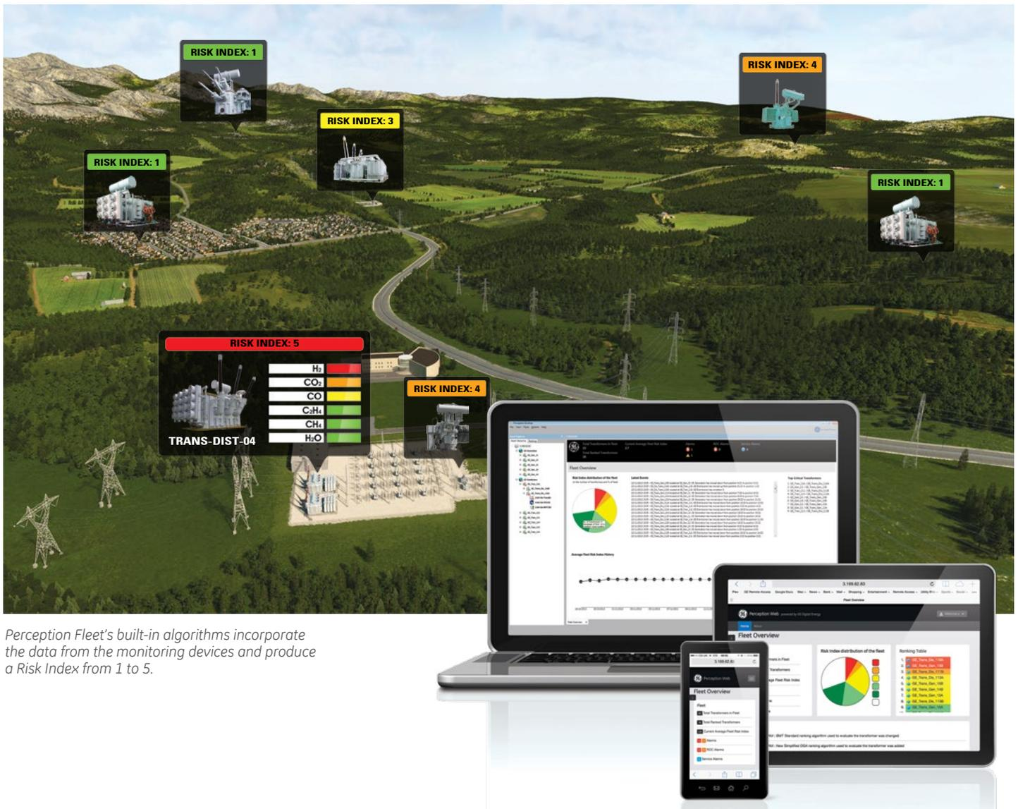
Perception Fleet's built-in algorithms incorporate the data from the monitoring devices and produce a Risk Index from 1 to 5.
