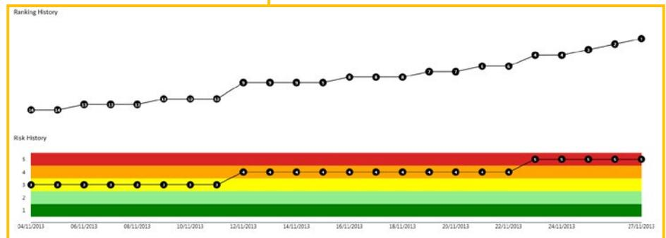
At the top the ranking history graph displays the transformers ranking position over a 30 day period. A condition statement for each point is displayed on the dashboard when a point is selected on the graph. The condition statement provides details on the risk and rank evaluation. At the bottom the risk history graph displays the transformer risk variation over a period of 30 days.
